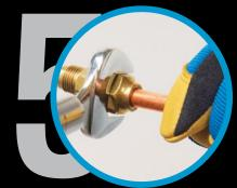
Thread the flare nut onto the male fitting and tighten using correct tools to equipment manufacturer torque specifications.
