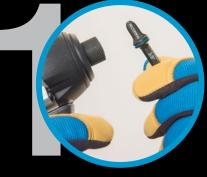
Choose bit size & attach it to the chuck or coupler. Fasten it well. Set power tool to MAX speed & torque if it is adjustable.
