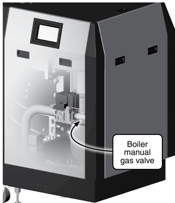
Figure 3 Boiler manual gas valve location, left-hand boiler configuration, front-mounted display (display may be in alternate location on the burner end access panel)
